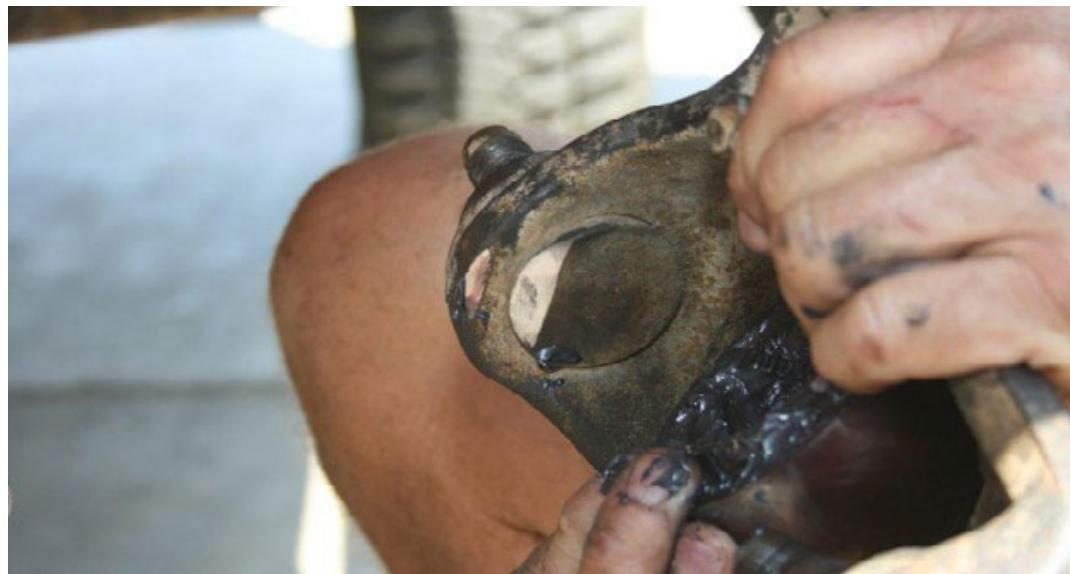
3. Once anything that needed to be modified, has been modified, the inner axle shaft can be inserted into the differential. Make sure that the axle shaft is fully inserted into the differential. This can be done by trying to rotate the axle shaft its self once it is believed to be seated. If the axle shaft has resistance to turning it is fully engaged into the differential.
