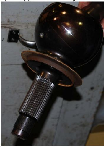
13. Sand the inside of the knuckle with fine sandpaper to remove all rust and other contaminates.
