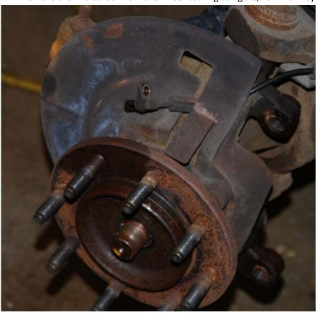
8. Unbolt the 4 unit bearing bolts with an 18mm socket.
