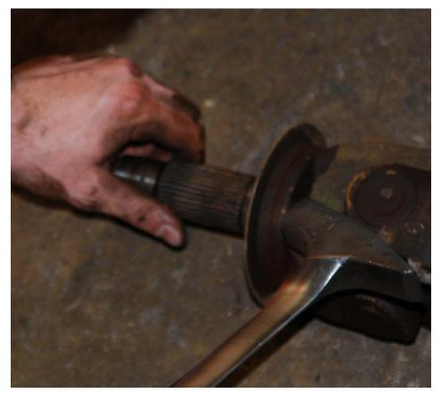
12. Install the bearing flange on the new RCV Performance axle. If the bearing flange is extremely rusty use sand paper to clean off the mating surfaces.
