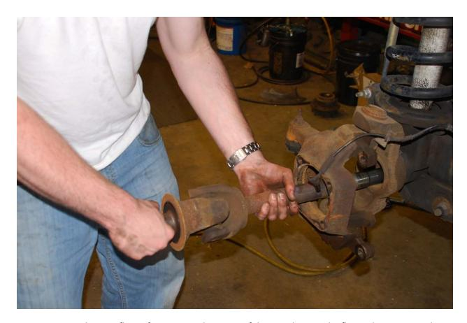
11. Remove bearing flange from OEM Axle. Be careful not to damage the flange during removal.
