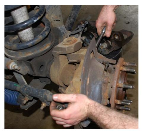
9. Remove the wheel bearing assembly and dust shield. A large hammer may be required if rust is present.
