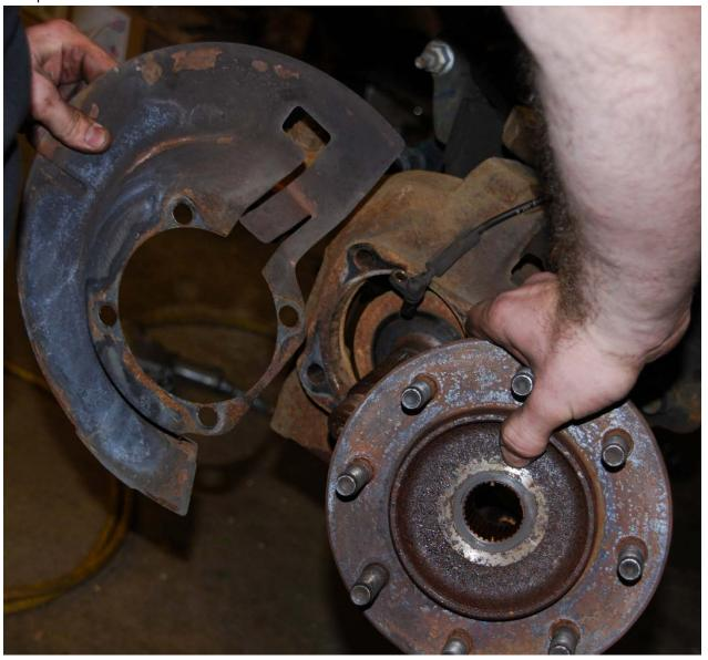
10. Remove OEM axle by pulling it straight through the knuckle.
